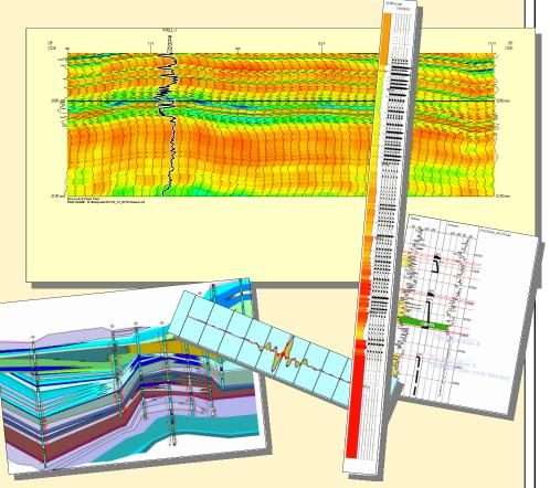
The conventional "Geological Cross Section" plots are limited, when someone wants to enter into small details. The reason is the "sampling rate". The popular rule tells that you have to take at least two samples from every wave, when you try to digitize a curve.
