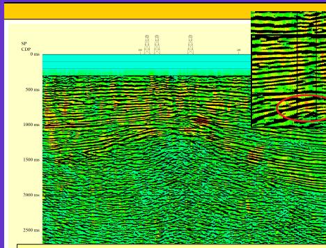
Seismic sections crossing well known gas fields.
