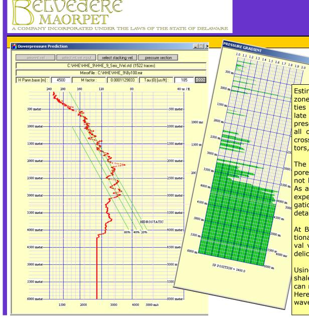
Estimating pore pressures and predicting over pressured zones on the basis of seismic wave propagation velocities is an old story. We started to study this topic at the late seventies, when the first international articles were presented. Soon it became an industry standard method all over the World. It has been tested several times, cross checked with actual mud weights and other indicators, such as drill head advancement ... etc.
